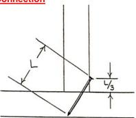
Note: The withdrawal value is taken from the lowest performing species of wood between the rafter and the top plate. For example, if the truss is Southern Pine and the wall top plates are Spruce-Pine-Fur, then the withdrawal value for the nails would be taken from the values for SPF.
