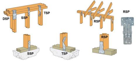
SST Solution: DSP, SSP, TSP, RSP (stud-to-plate ties) Literature: C-C-2021, pp. 280-282
