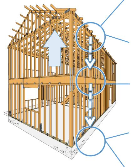
Starting at the top of the structure, forces are transferred from the roof truss or rafter to the top plate of the wall
