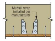
MASA(P) installed on the same side as the sheathing
